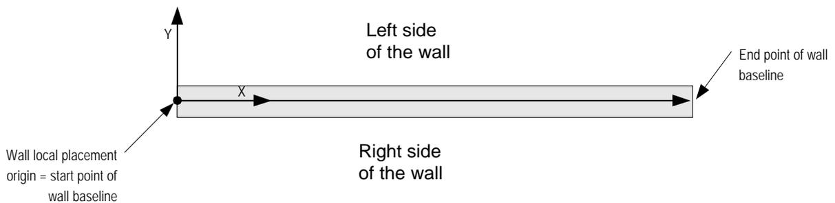
The second solution would be to use the local placement of IfcDoor itself. The IfcOpeningElement containing IfcDoor is placed relative to IfcWall, and IfcDoor is placed relative to IfcOpeningElement. The direction of the local coordinate system of IfcDoor would decide what is left and what is right.
