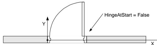
The second solution is to always place the local coordinate system origin on the side of the hinge and omit the HingeAtStart attribute.
